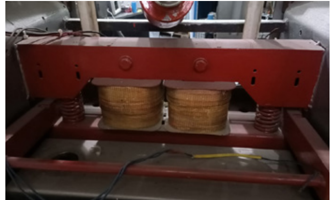
Solenoid/contactator type actuator.
